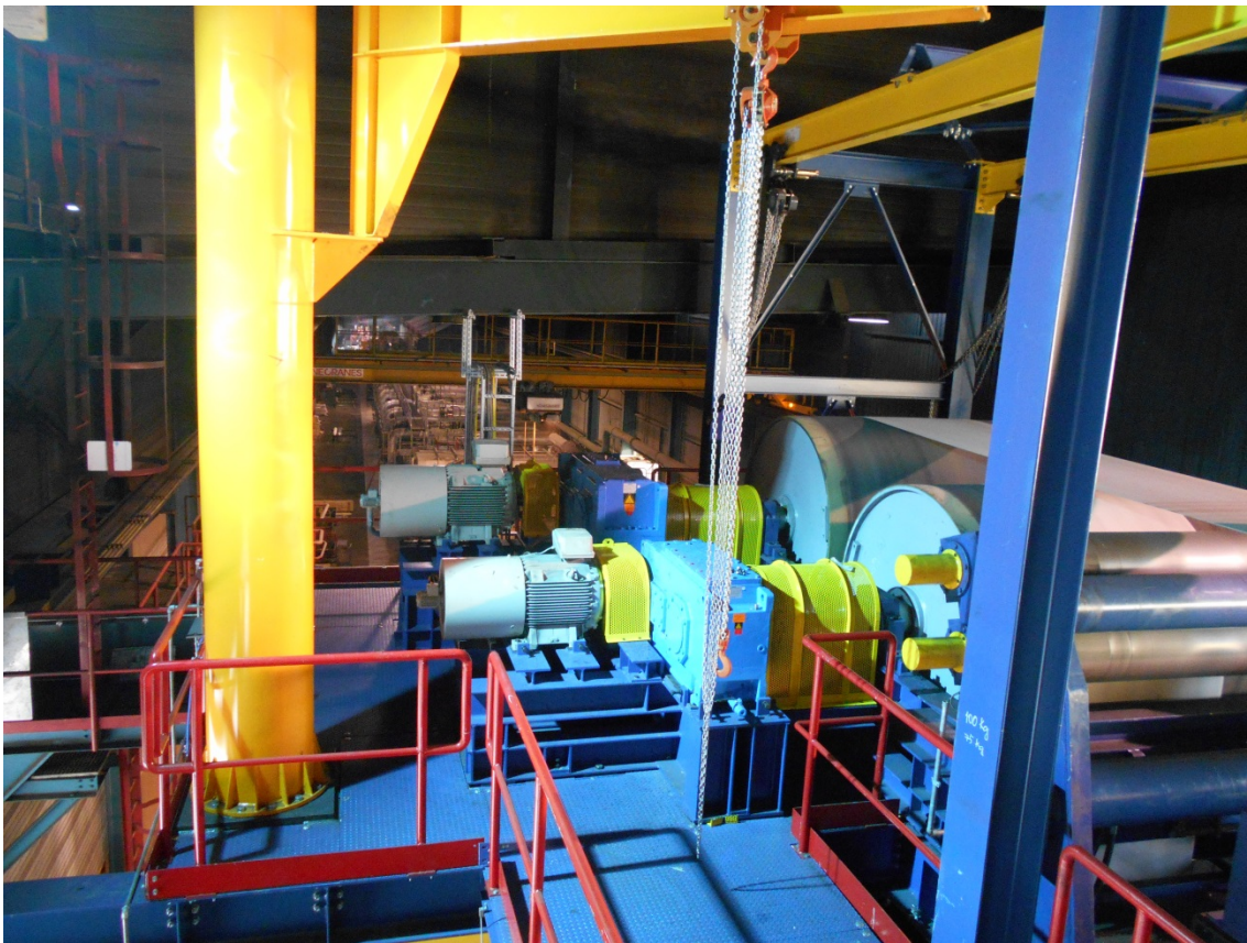
Modernized bridle area of the annealing and pickling line of Aperam in Genk in Belgium which was modernized by Primetals Technologies
