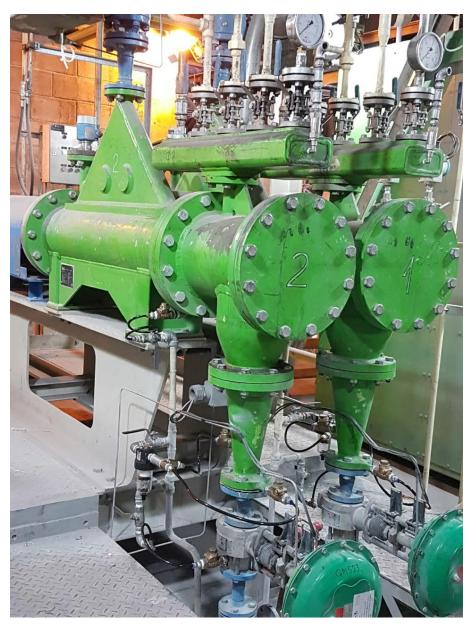
Volumetric dosing device for precise feeding of Mg with rates between 3 and 15 kg/min
