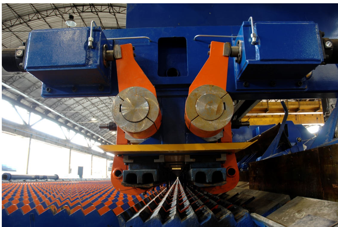
High-speed delivery system of a bar mill from Primetals Technologies
