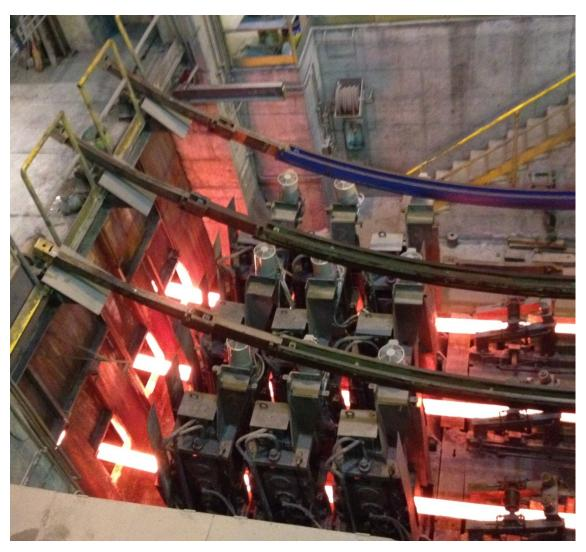
Three-strand continuous billet caster from Primetals Technologies at the Bolzano plant site of Italian steel producer Acciaierie Valbruna S.p.a.
