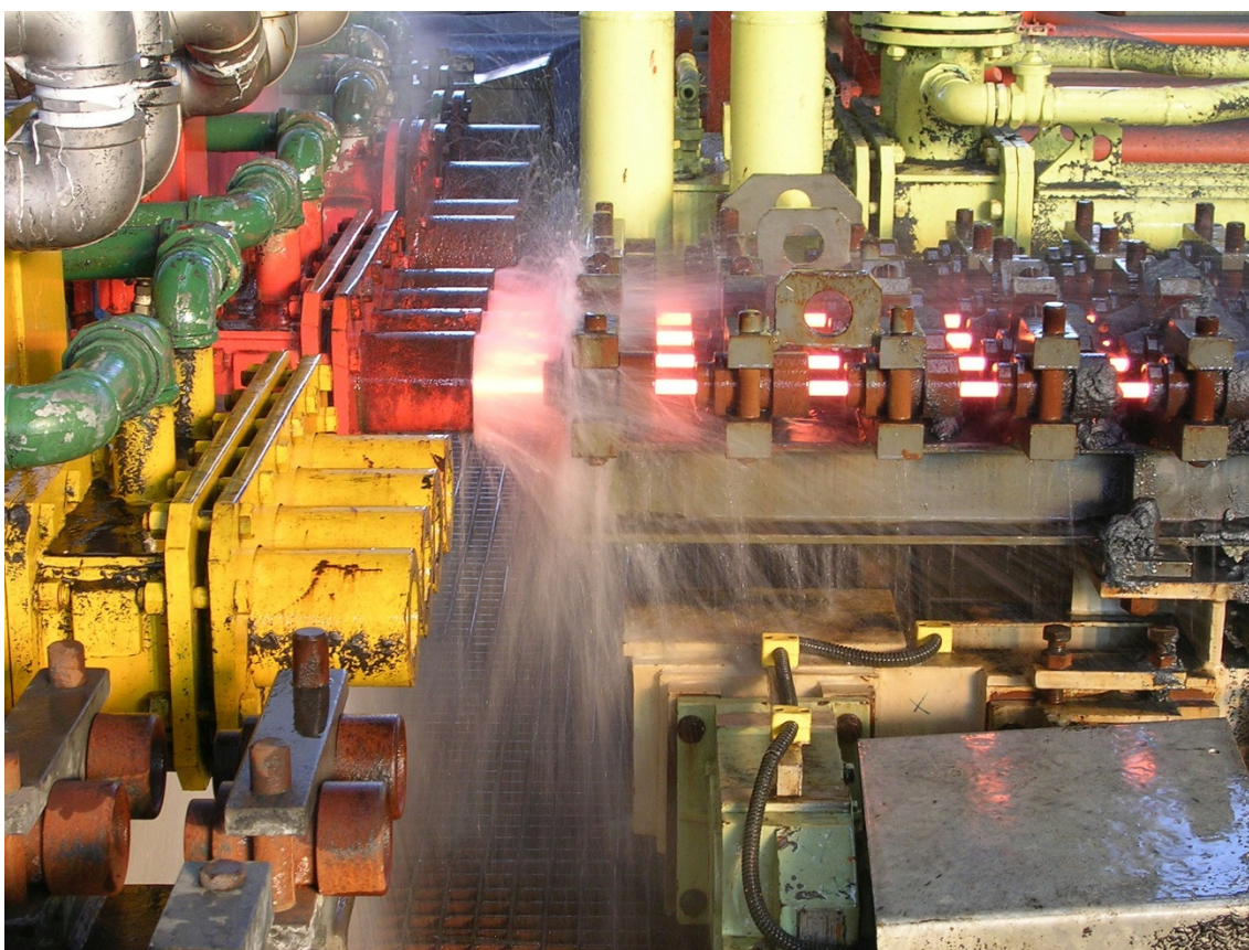
PQS heat-treatment system in multi-slit operation in a bar mill from Primetals Technologies
